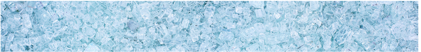
Fine crumbly breakage of toughened safety glass.
